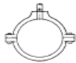
FIG. 41 - Page 30 SPLIT RING EXTENSION HANGER WW-H-171-E TYPE 25 A-A-1192 A TYPE 12 MSS SP-58 and SP-69 TYPE 12
