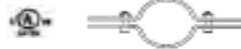
FIG. 50 - Page 35 RISER CLAMP WW-H-171-E TYPE 8 A-A-1192 A TYPE 8 MSS SP-58 and SP-69 TYPE 8
