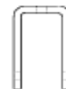
FIG. 86 - Page 45 WELDING BEAM ATTACHMENT WITH AND WITHOUT BOLT WH-H-171-E TYPE 22 A-A-1152 A TYPE 22 MSS SP-58 and SP-69 TYPE 22
