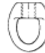
FIG. 47 - Page 33 EYE SOCKET WW-H-171-E TYPE 16 A-A-1192 A TYPE 16 MSS SP-58 and SP-69 TYPE 16
