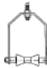
FIG. 272SS - Page 87 ADJUSTABLE ROLLER HANGER, STAINLESS STEEL WW-H-171-E TYPE 44 A-A-1192 A TYPE 43 MSS SP-58 and SP-69 TYPE 43
