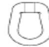
FIG. 13, 13I & 13L - Page 18 WELDLESS EYE NUT WH-H-171-E TYPE 17 A-A-1152 A TYPE 17 MSS SP-58 and SP-69 TYPE 17
